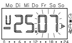
The **+** and **-** keys can now be used to change the month (flashing).
