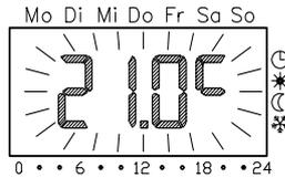
This can now be changed with the + and - keys. Pressing the SET key confirms the set new temperature. The temperature is regulated to this value until the next switching time of the time program at which time the temperature of the time program is resumed.
